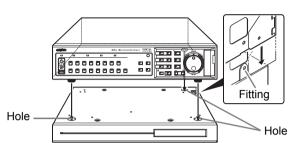
(2) Use the remaining screw (accessory) to secure the fitting on to the right side of the DVR. Tightening torque: 0.6 N•m - 0.7 N•m
